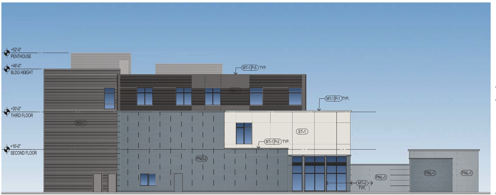
ELEVATION - WEST (ALLEY) SCALE: 3/32" = 1'-0"
