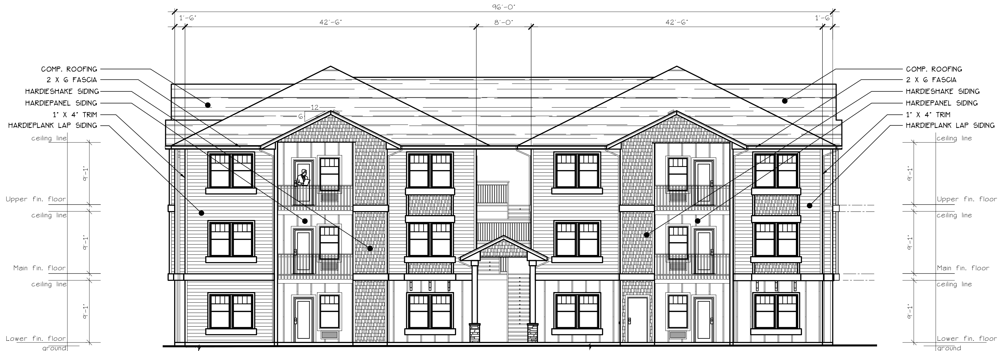
NORTH ELEVATION (BLD. 27+31) SCALE: 1/8" = 1'-0" TYPE E UNIT
