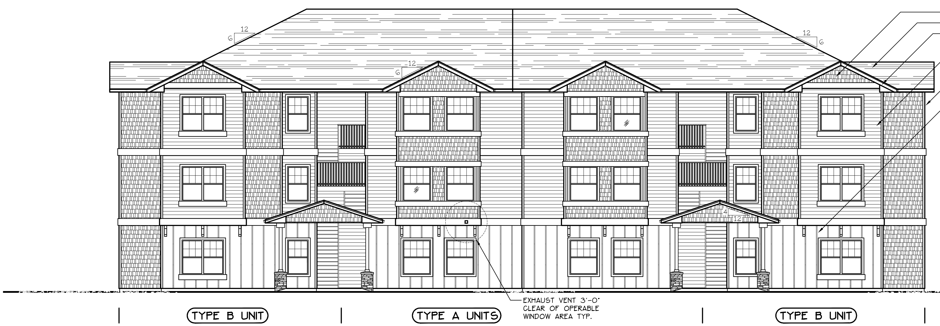
FRONT ELEVATION (BLD. 23+35) SCALE: 1/8" = 1'-0"
