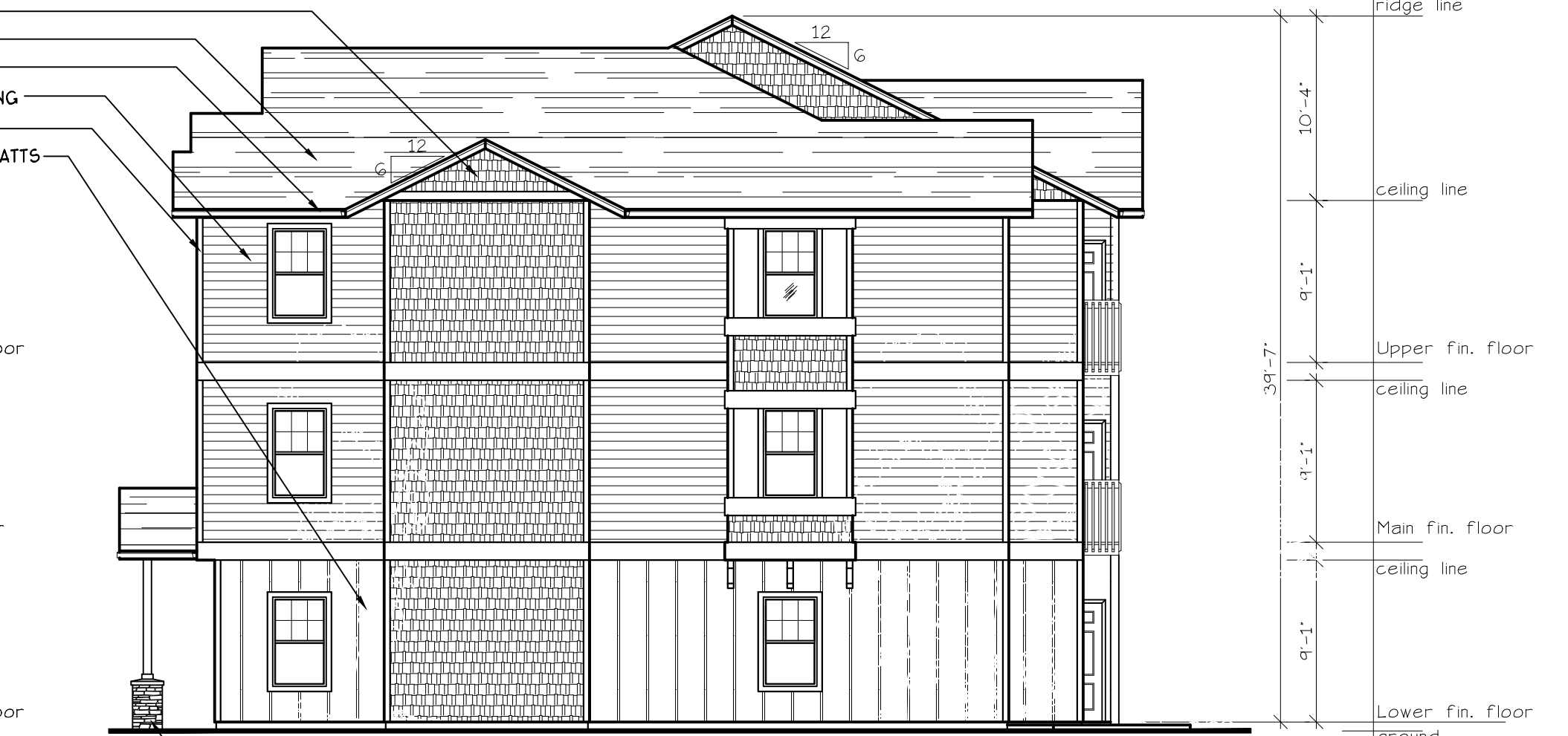
SIDE ELEVATION (BLD. 20.32+34) SCALE: 1/8" = 1'-0"
