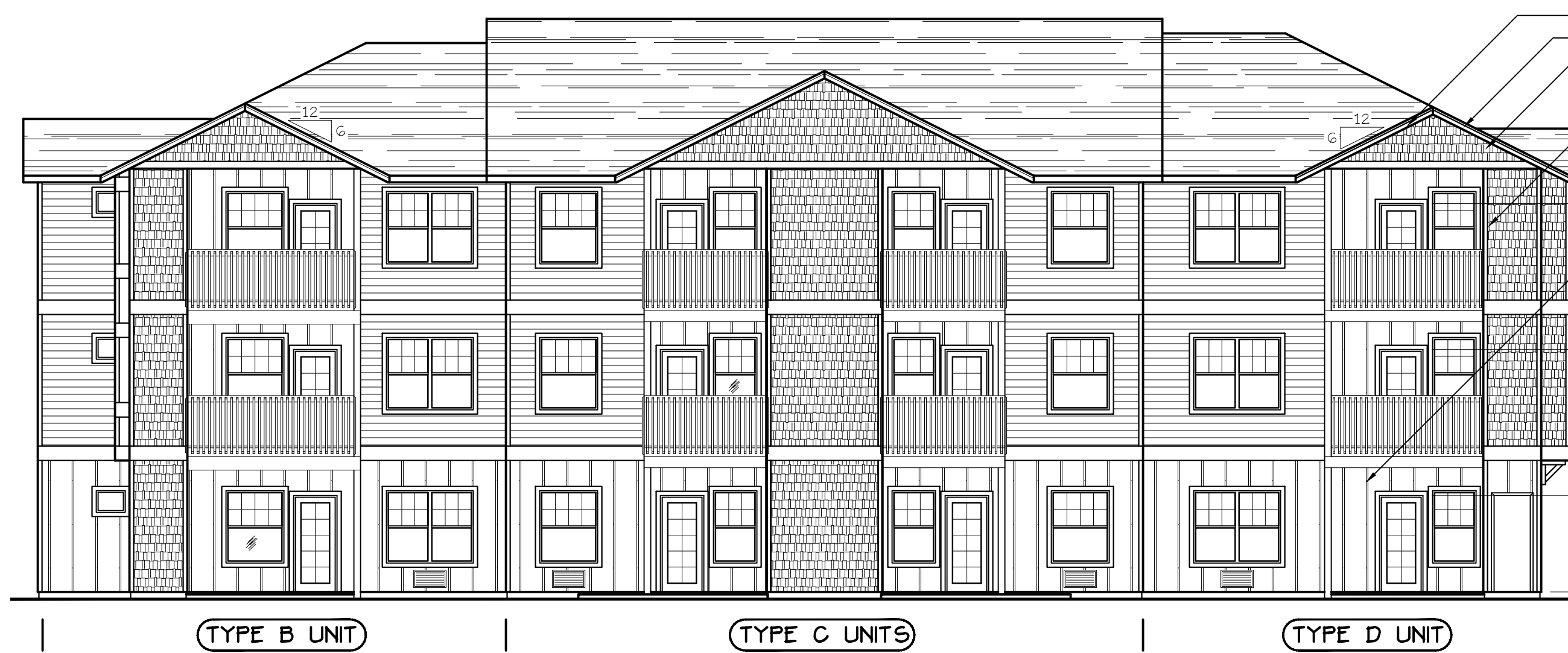
TYPE B UNIT | TYPE C UNITS | TYPE D UNIT SOUTH ELEVATION (BLD. 22) SCALE: 1/8" = 1'-0"
