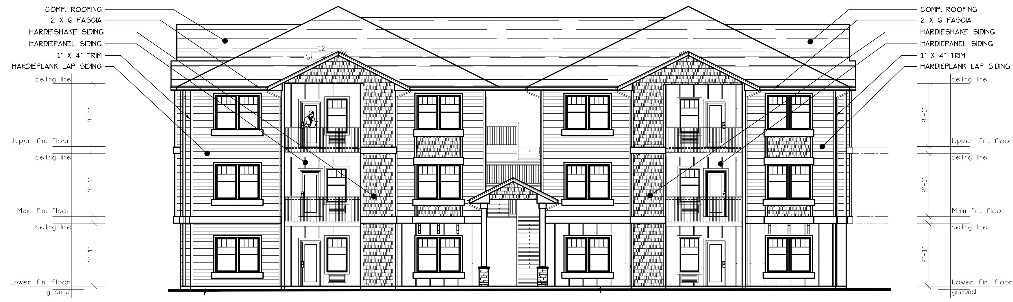
SOUTH ELEVATION (BLD. 27+31) SCALE: 1/8" = 1'-0" TYPE E UNIT
