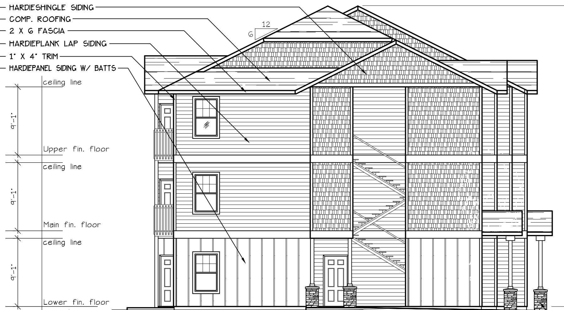
END ELEVATION (TYPE A UNITS) SCALE: 1/8" = 1'-0" BLD. 21+29
