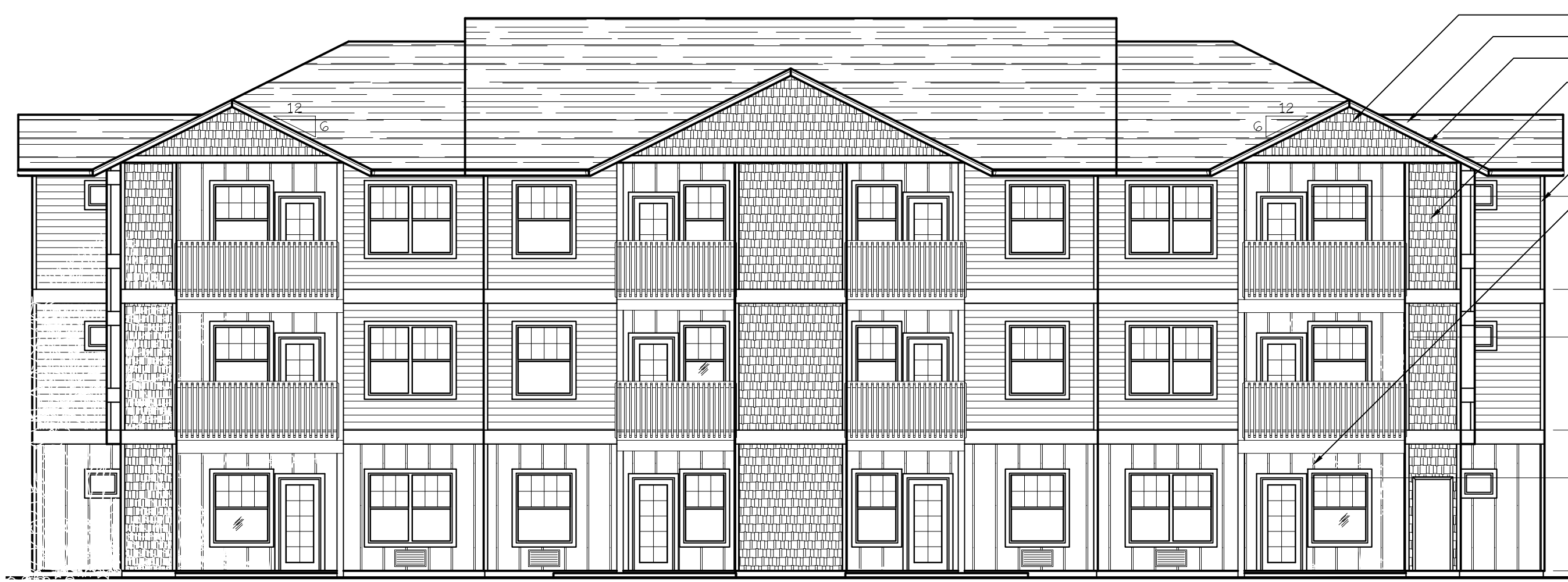
REAR ELEVATION (BLD. 20.32+34) SCALE: 1/8" = 1'-0"
