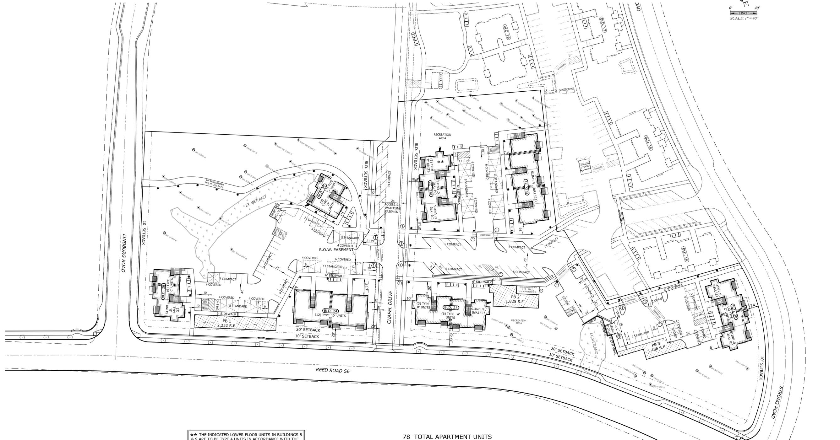
★★ THE INDICATED LOWER FLOOR UNITS IN BUILDINGS 5 & 9 ARE TO BE TYPE 'A' UNITS IN ACCORDANCE WITH THE 2014 OSSC SEC. 1107.6.2.1.1 (NOTED ON FLOOR PLANS). ALL OTHER LOWER FLOOR UNITS TO BE TYPE 'B' UNITS IN ACCORDANCE WITH THE 2014 OSSC SEC. 1107.6.2.1.2
