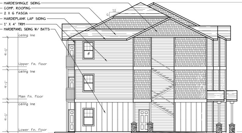
END ELEVATION (TYPE A UNITS)
