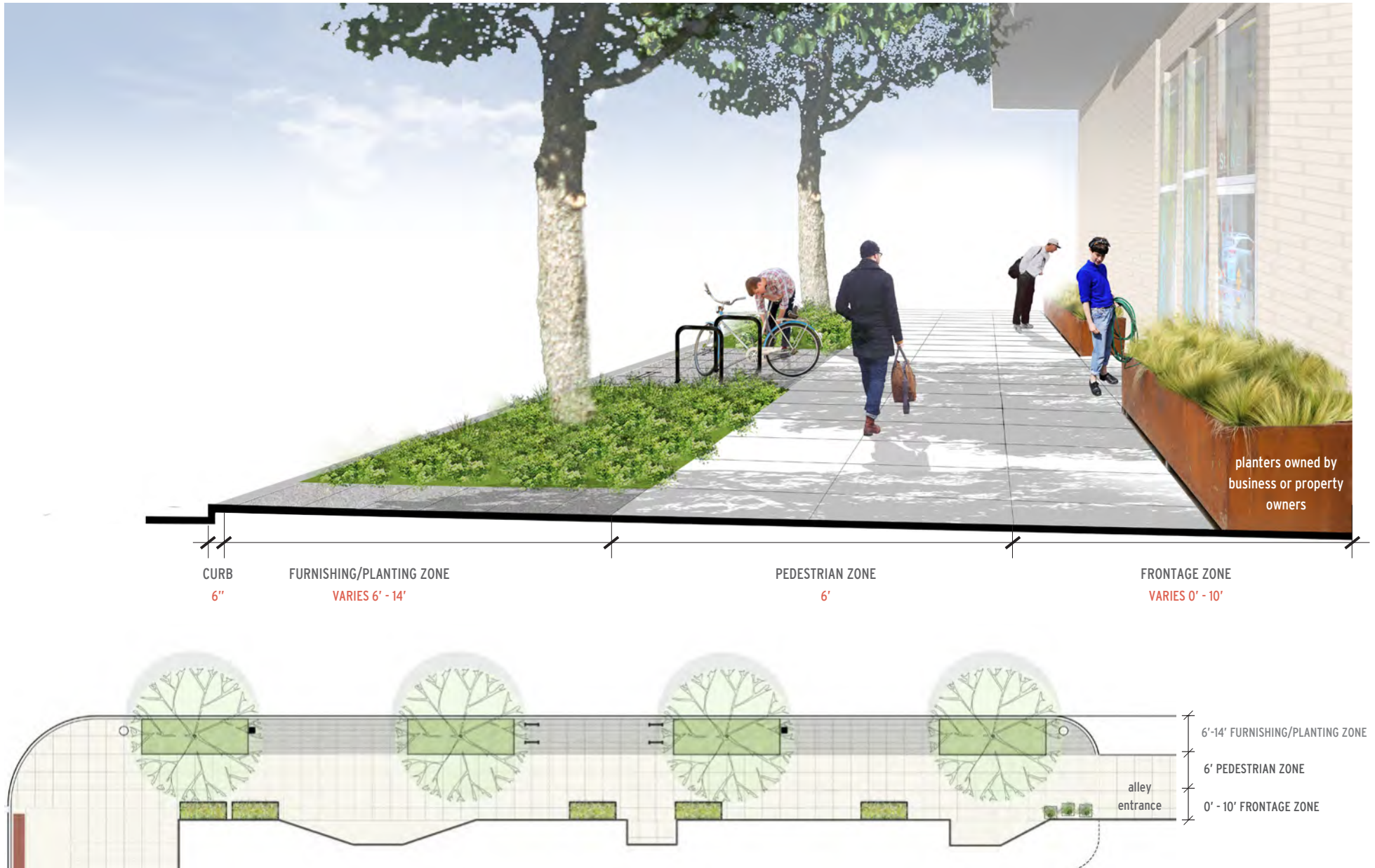
This plan shows an example of one half-block, from a corner to the middle of the block.
