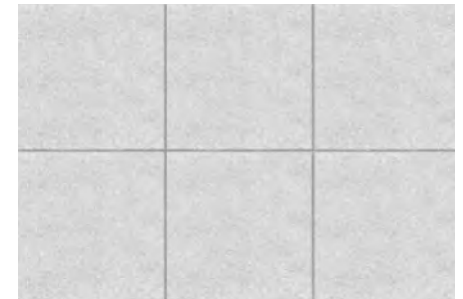
FRONTAGE ZONE AND PEDESTRIAN ZONE, SIMPLE CONCRETE, 3'X3' SCORING GRID
