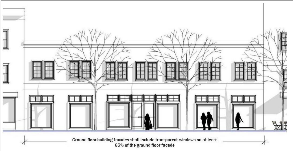
FIGURE 533-5 GROUND FLOOR WINDOWS
