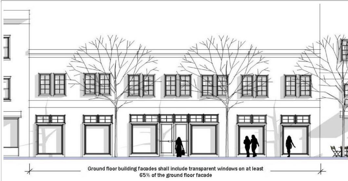
FIGURE 533-5 GROUND FLOOR WINDOWS
