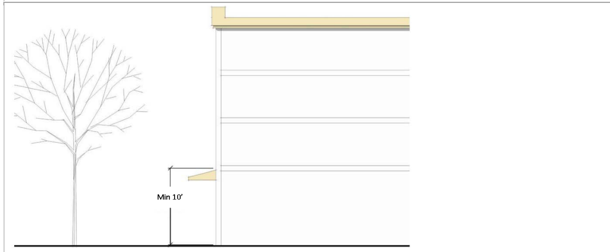
FIGURE 536-2 GROUND FLOOR HEIGHT
