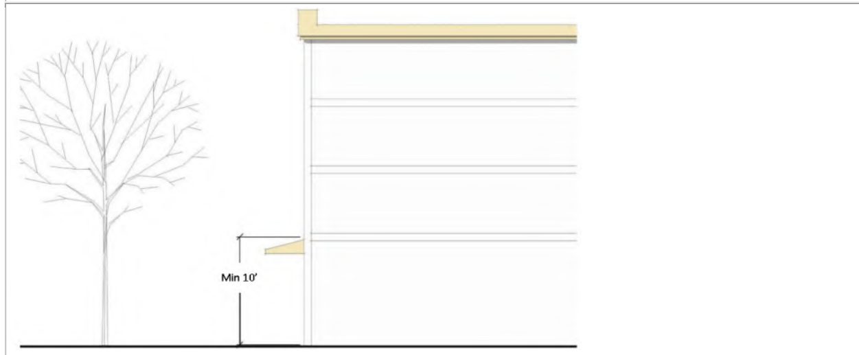
FIGURE 536-2 GROUND FLOOR HEIGHT
