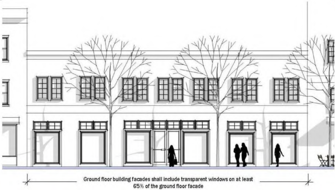
FIGURE 536-5 GROUND FLOOR WINDOWS
