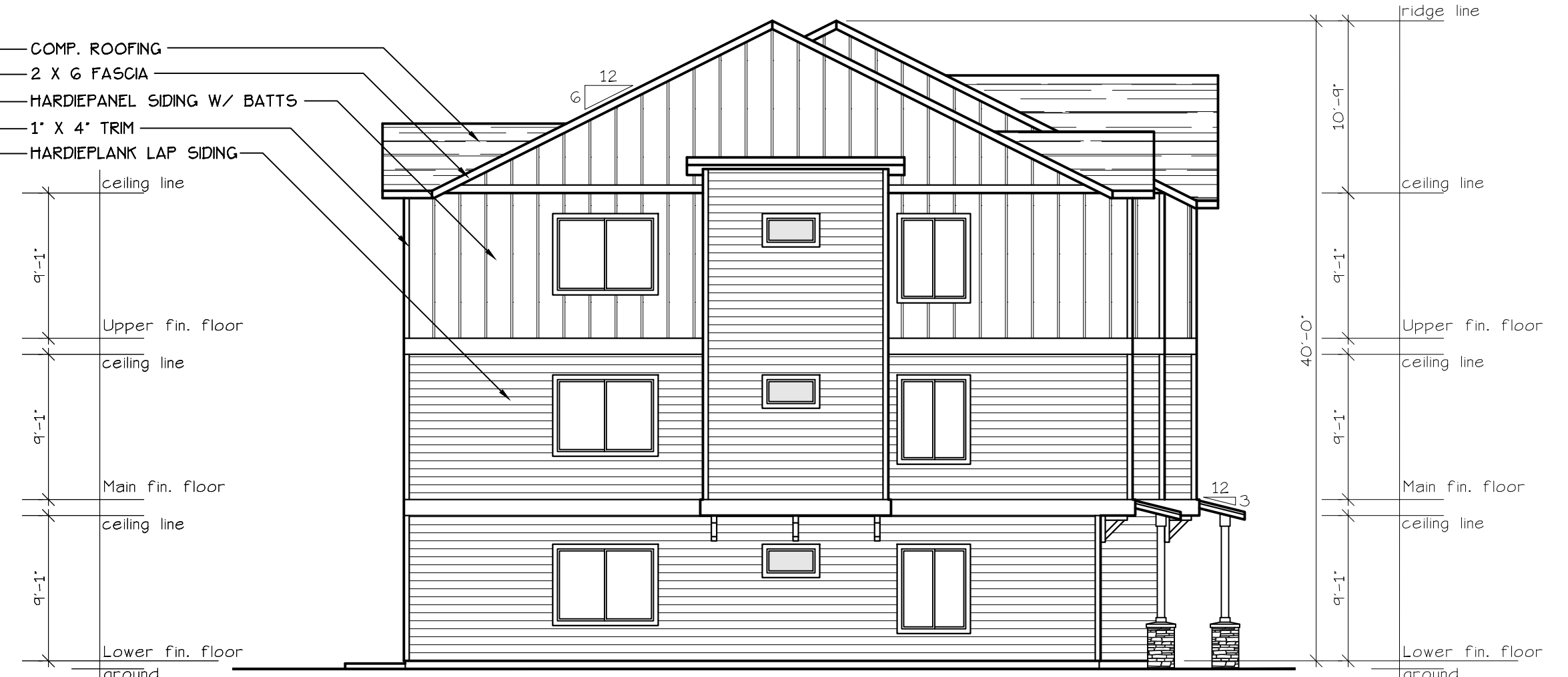
END ELEVATION (TYPE A UNITS) SCALE: 1/8" = 1'-0" BLD. 3.4.6.10-14.16.17.20.25.31+32
