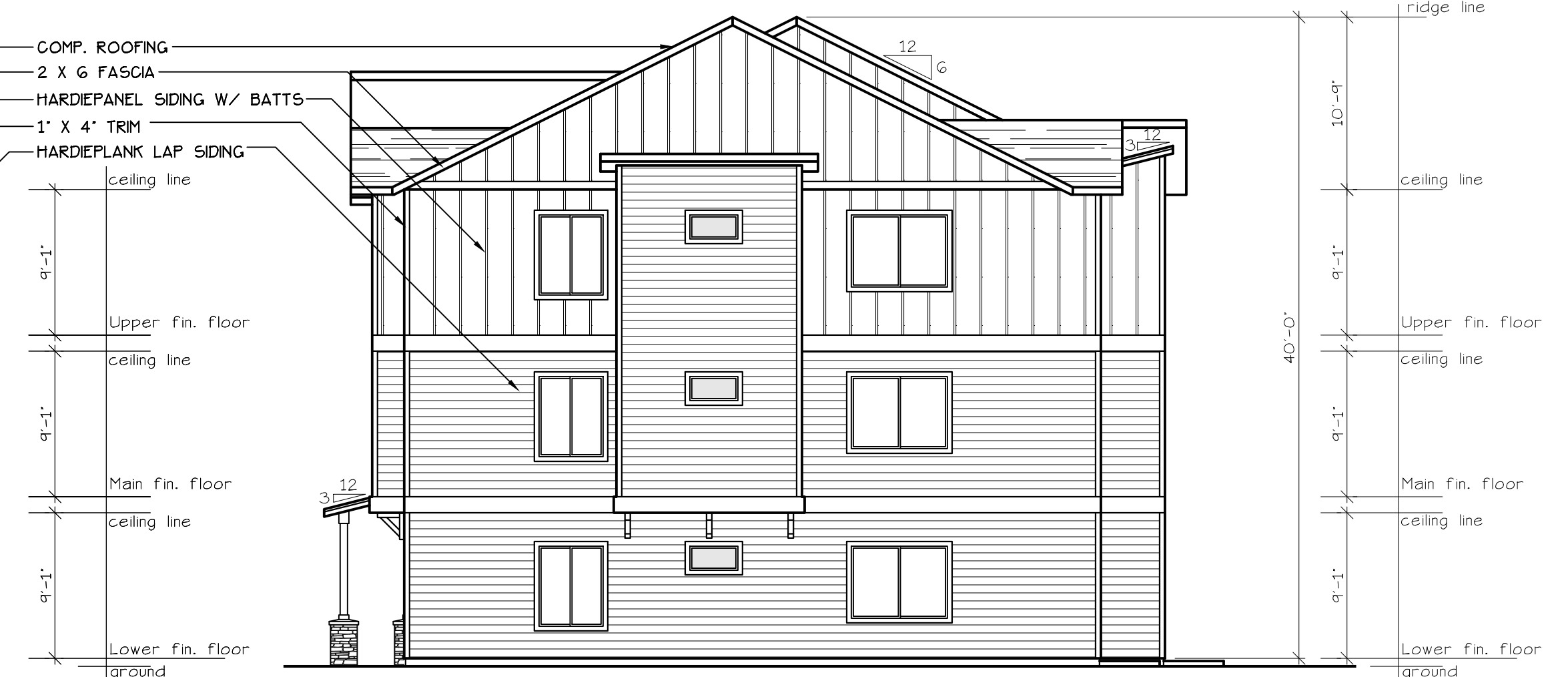
END ELEVATION (TYPE A UNITS) SCALE: 1/8" = 1'-0" BLD. 3.4.6.10-14.16.17.20.25.31+32
