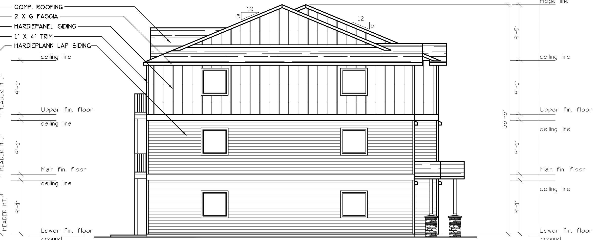
NORTH ELEVATION (TYPE B UNITS) SCALE: 1/8" = 1'-0" BLD. 13,19,23,26,+29
