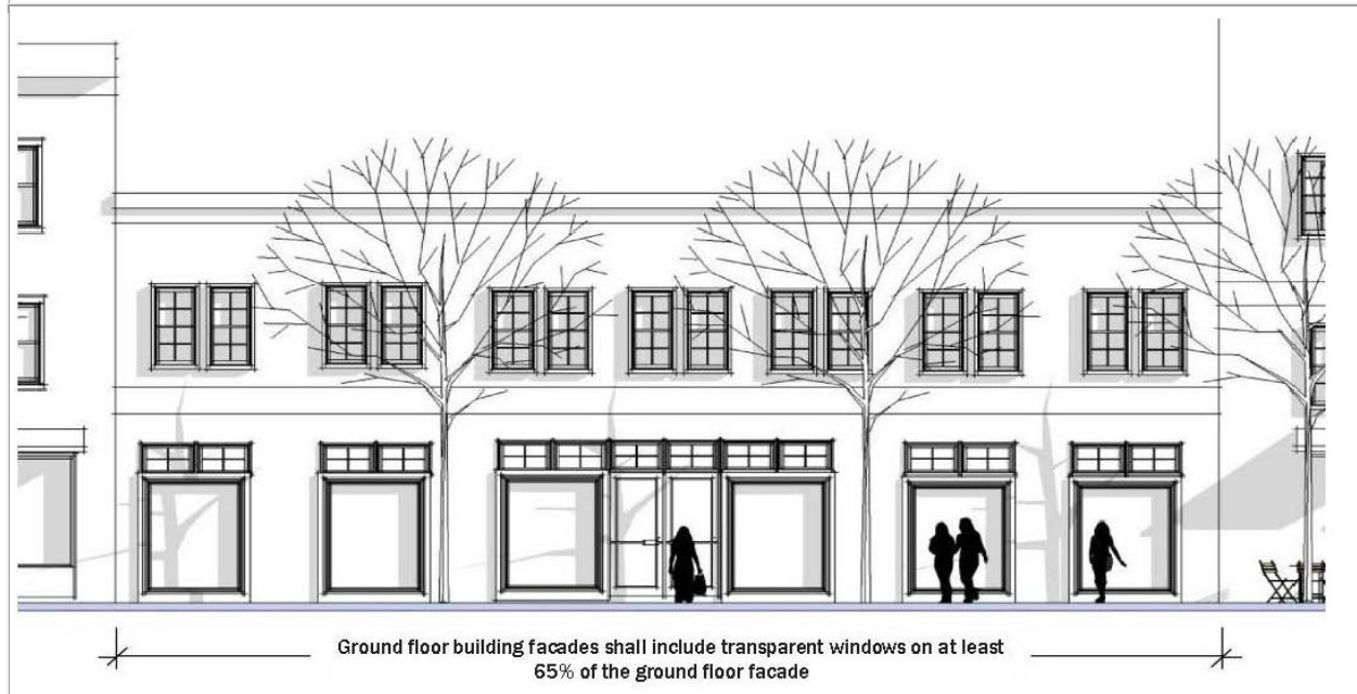
FIGURE 533-5 GROUND FLOOR WINDOWS
