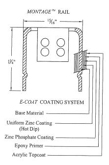
RAKING DIRECTIONAL ARROW Welded panel can be raked 45" over 8' with arrow pointing down grade. PROFUSION "WELDING PROCESS No exposed welds. Good Neighbor profile - Same MONTAGE RAIL appearance on both sides Specially formed high strength architectural shape.
