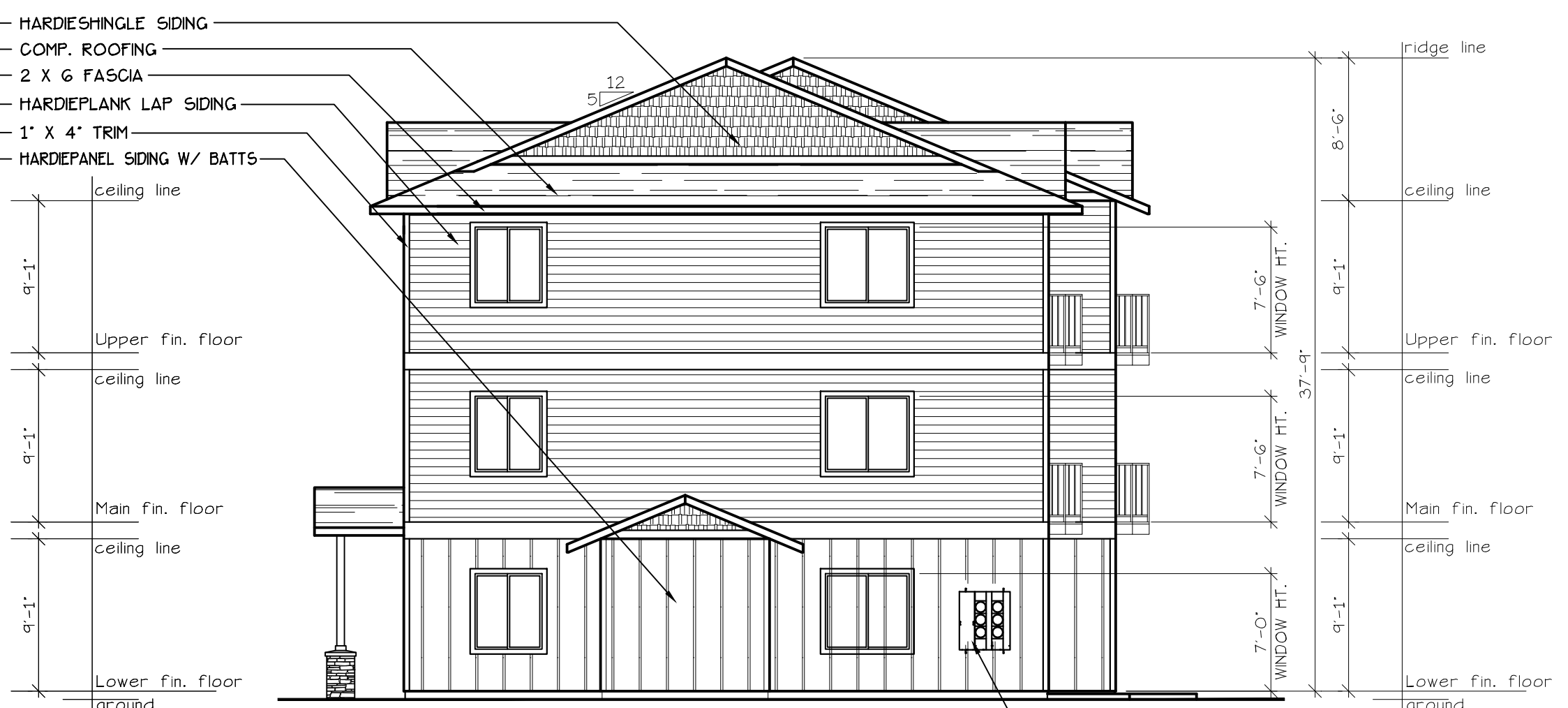
NORTH ELEVATION (TYPE A UNITS) SCALE: 1/8" = 1'-0" BLD. 2
