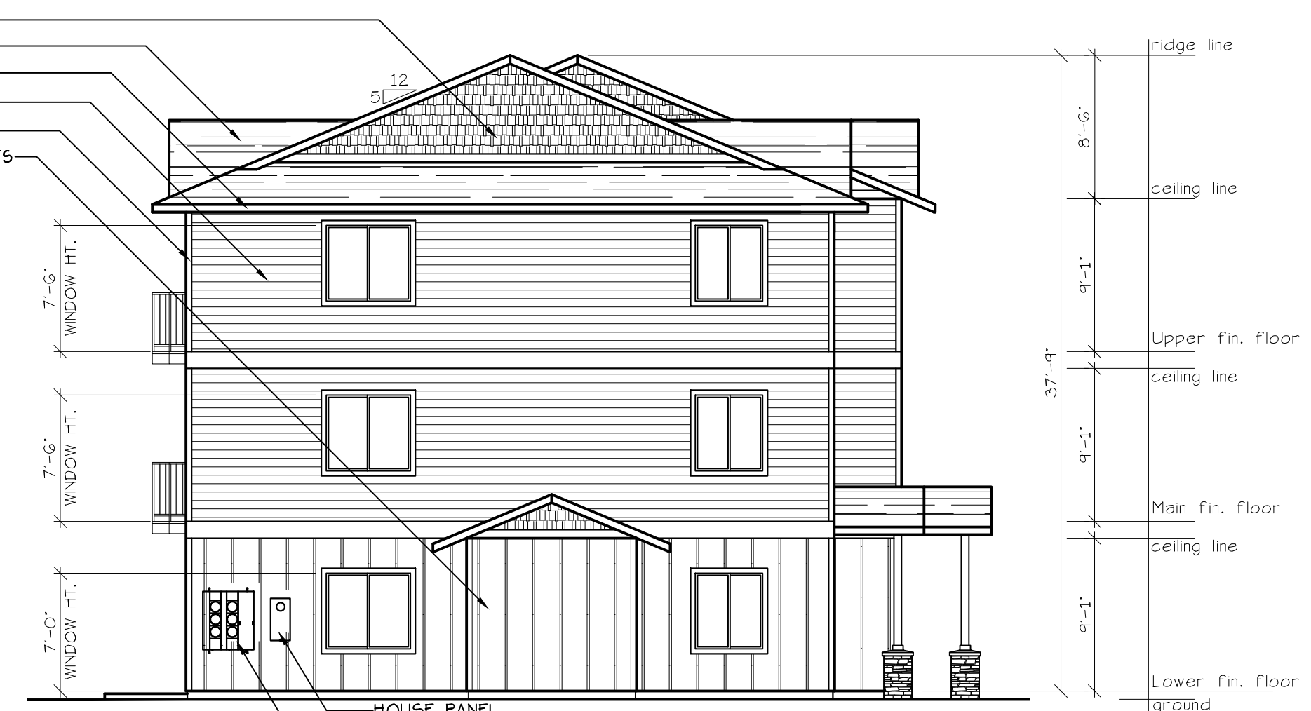
SOUTH ELEVATION (TYPE A UNITS) SCALE: 1/8" = 1'-0" BLD. 2
