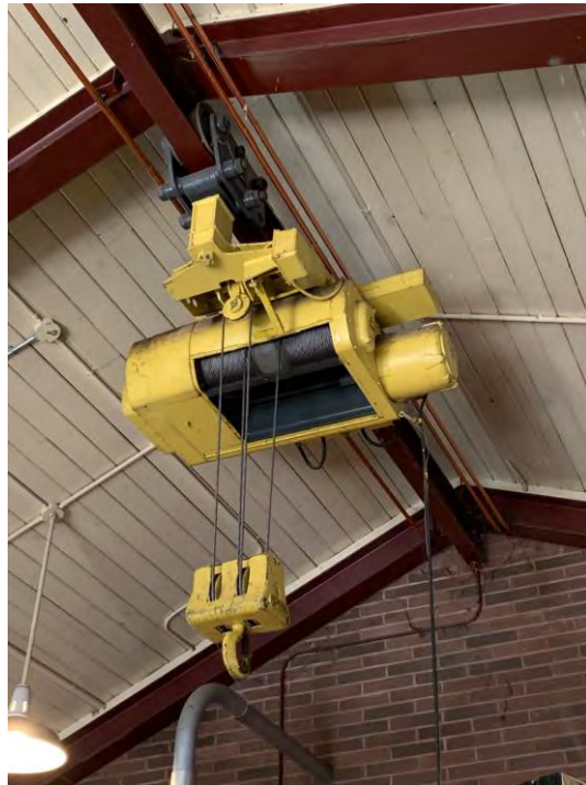
Figure 3.69 Unrestrained Overhead Bridge Crane
