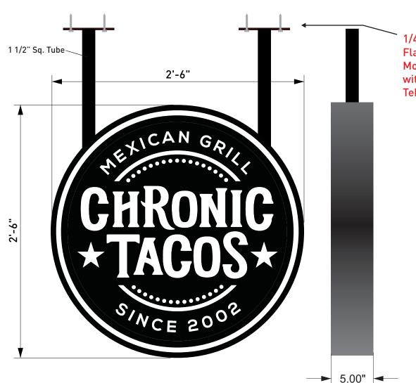
1/4" x 1 1/2" x 6" Flat Stock Metal; Mounted to canopy with eight (8) 1/4" x 2" **Tek Screws**
