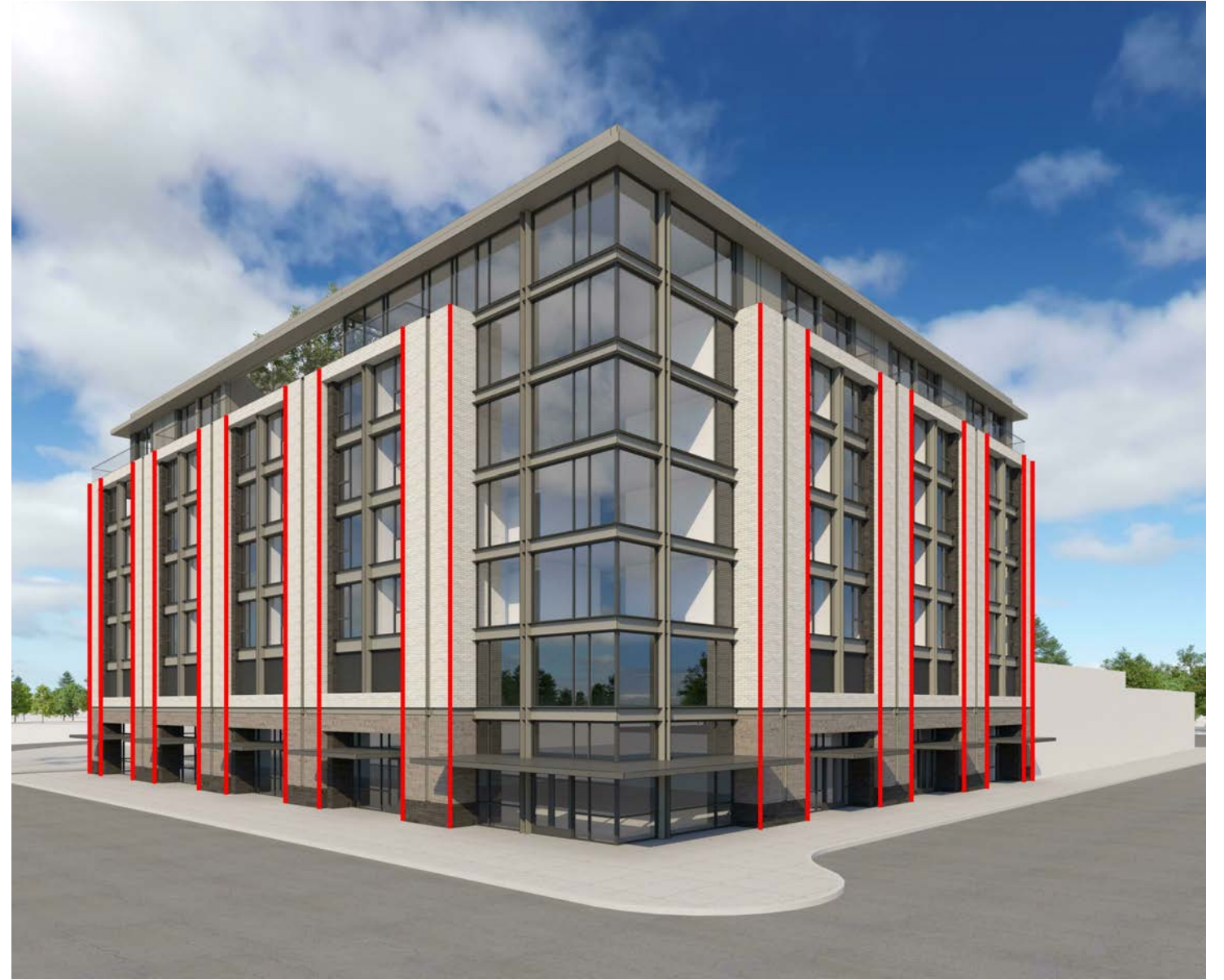
PROPOSAL: VERTICAL MASONRY PIERS AND GROUPED WINDOWS
