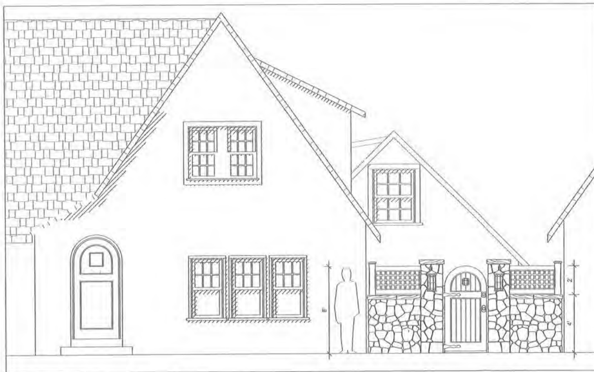
1 Elevation - Stone Wall and Gate Scale: 1/4" = 1'-0"
