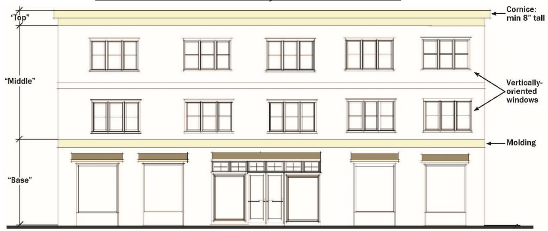
FIGURE 524-2. BUILDING FAÇADE ARTICULATION
