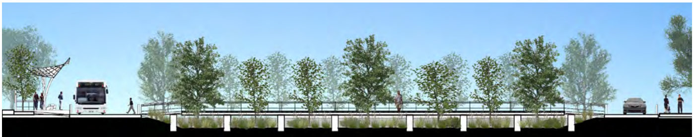
Figures 42 - 44. Cross-sections: Bus station; Bioswale boardwalk; Bioswale.
