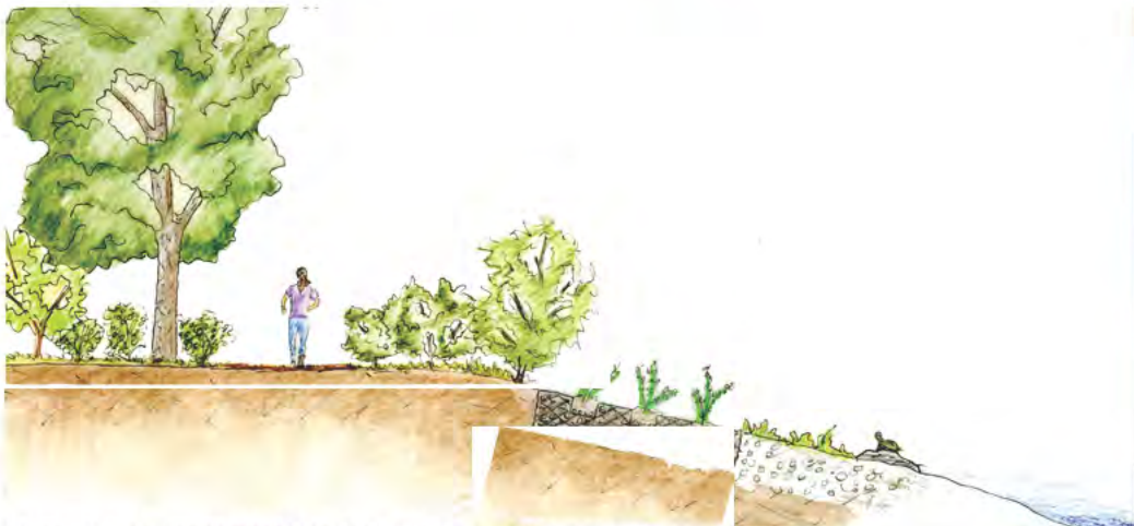
Figure 25. Proposed restoration: gabion-modified slough bank.
