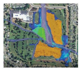
Figure 5.10: Revised detention areas (orange) at peak of modeled 100-year flood event (incorporated in Preferred Alternative)
