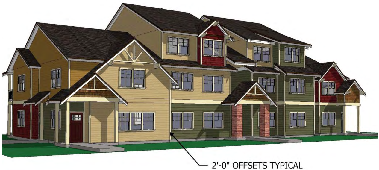
Figure 21A: Example Building Front Offset for refinement to DDH 2.E.4.b.1) as indicated in the above table
