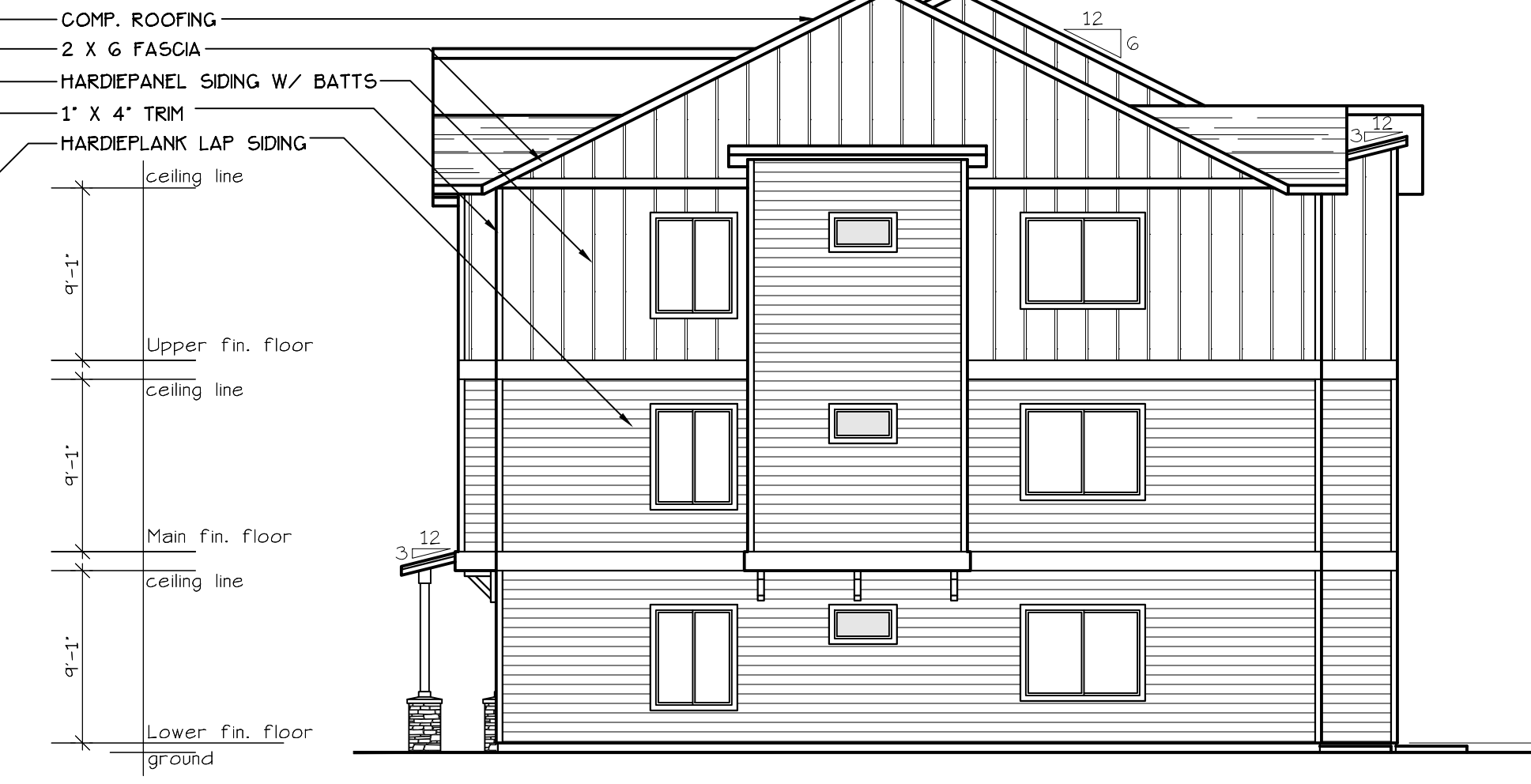
END ELEVATION (TYPE A UNITS) SCALE: 1/8" = 1'-0" BLD. 3.4.6.10-14.16.17.20+25
