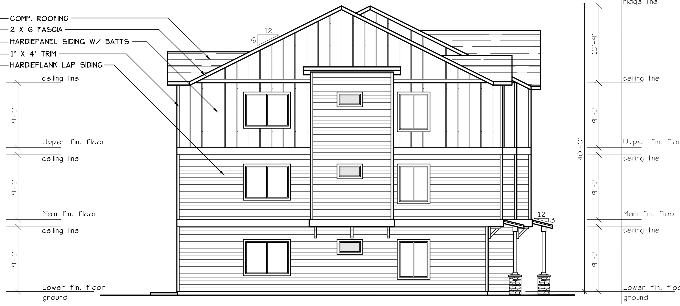
END ELEVATION (TYPE A UNITS) SCALE: 1/8" = 1'-0" BLD. 18
