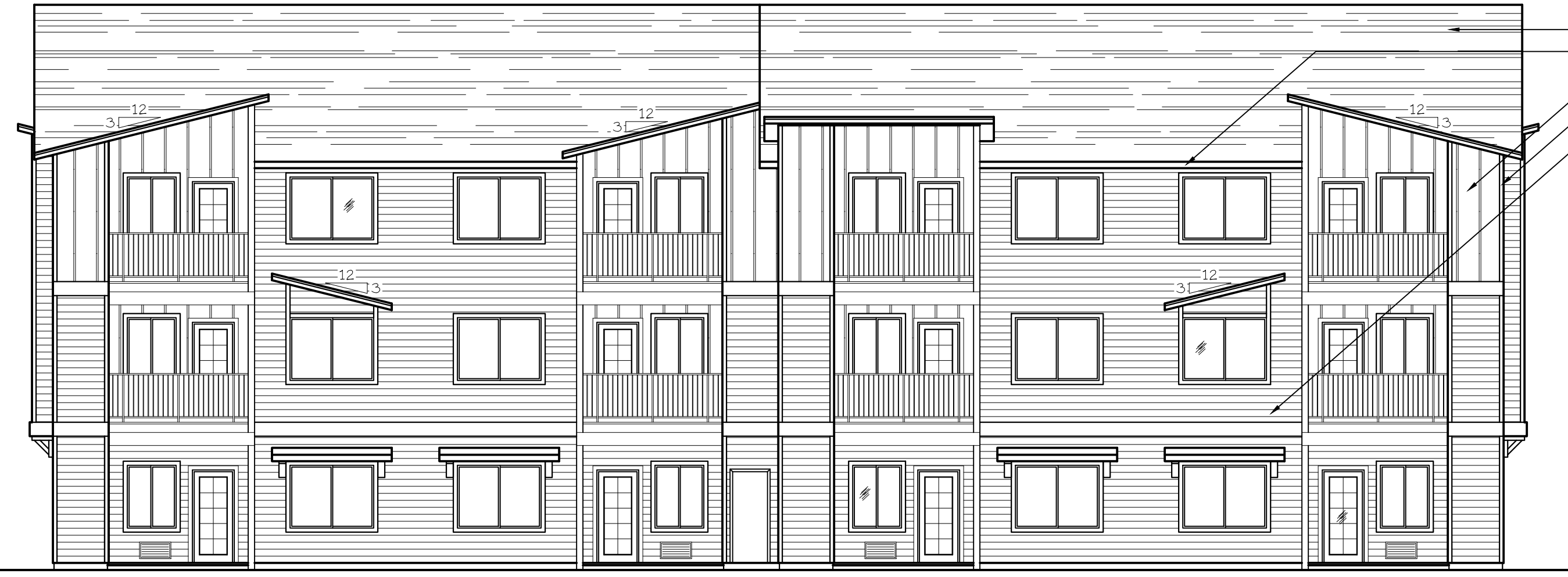
REAR ELEVATION (TYPE A UNITS) SCALE: 1/8" = 1'-0" BLD. 3.4.6.10-14.16.17.20+25
