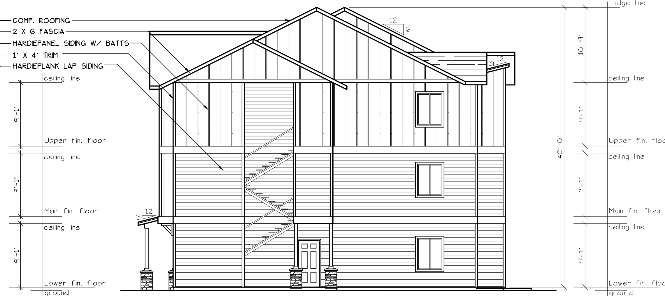
END ELEVATION (TYPE A UNITS) SCALE: 1/8" = 1'-0" BLD. 18
